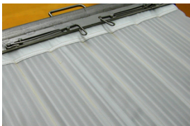
Diastar filter installed on filtrate drainage system
