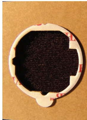
Filter component made of mesh-felt combination
