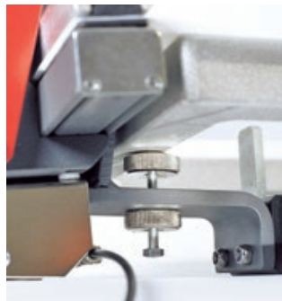
Frame profile height adjusting screw of SEFAR® 3A
